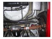
5. Install the passenger side tailpipe into muffler assembly using clamp #C to secure. Do not tighten. Use the stock clamp to secure the tailpipe to the stock h-pipe.
