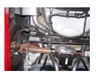
6. Now do the same procedure for the driver side tailpipe. Use clamp #C to secure the tailpipe to the muffler assembly and the stock clamp to secure it to the stock h-pipe.
